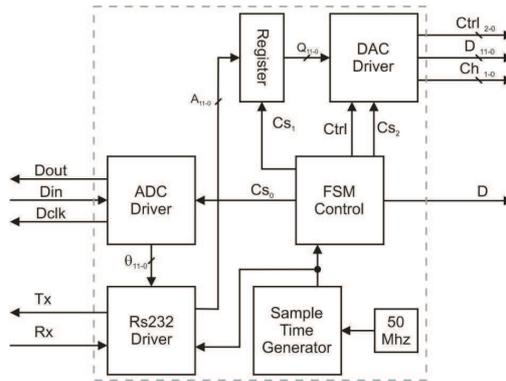
Fig. 7. Hardware description for FPGA block diagram.
