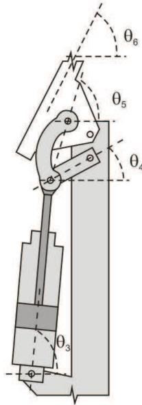
Fig. 1. Mechanical-Pneumatic system for the flexible manipulator.
