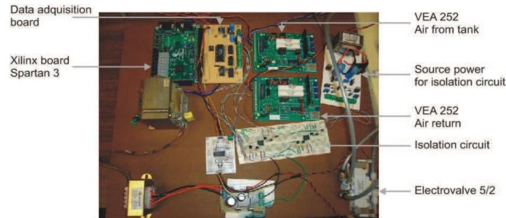
Fig. 9. Hardware used for flexible manipulator control.
