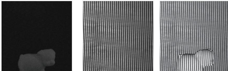
Fig. 3 (a) Mud pig; (b) Fringe pattern; (c) Fringe pattern over a mud pig.
