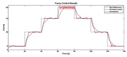
Fig. 10. Fuzzy control behavior of the flexible arm.
