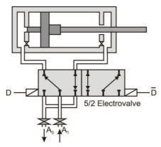
Fig. 2. Pneumatic system for the flexible arm manipulator.
