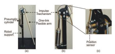
Fig. 8. Flexible manipulator robot prototype. (a) General view. (b) Impulse mechanism. (c) Position sensor.
