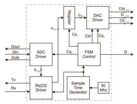
Fig. 7. Hardware description for FPGA block diagram.
