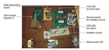
Fig. 9. Hardware used for flexible manipulator control.
