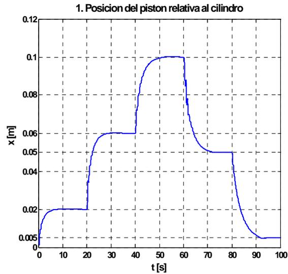
Figure 4. PID Controller result for the pneumatic system.
