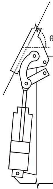
Figure 1. Mechanical-Pneumatic system for the flexible manipulator.
