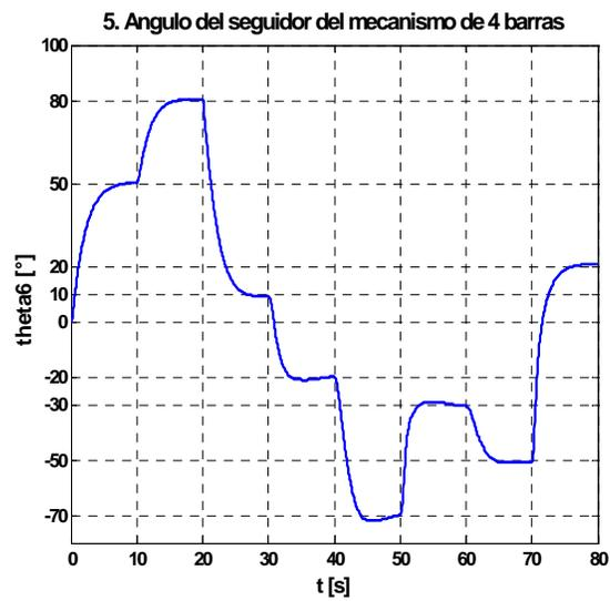
Figure 6. PID control position, to the output angle  $\theta$ , for the pneumatic-mechanical system.
