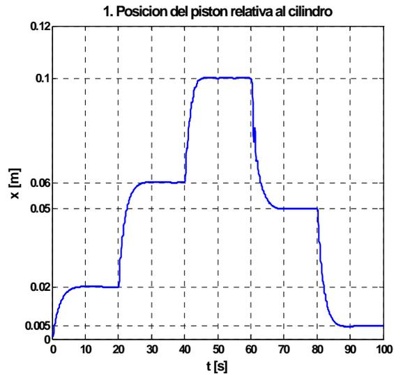
Figure 5. Pneumatic system with discrete PID controller.
