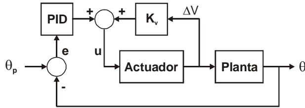
Figure 3. Position controller of flexible arm impulse mechanism with speed change feedback.
